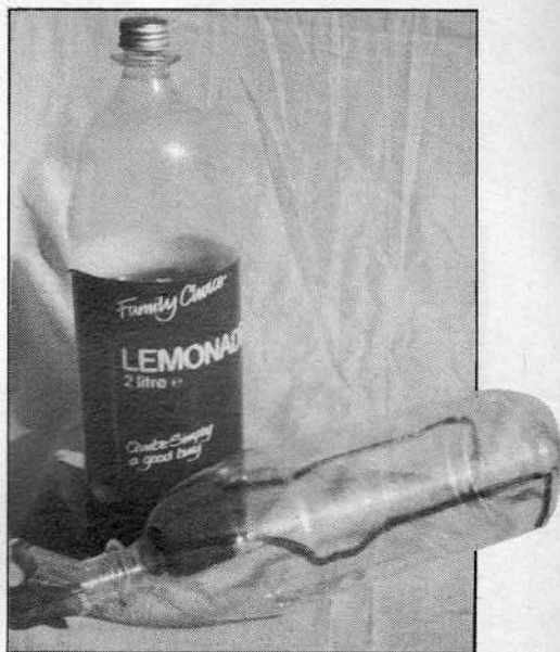
Above: the basis for Terry's DIY bodyshells; plastic drinks bottles. Mark out the shape using a 'Magic Marker' felt tip and then cut out with sharp scissors.
